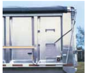
The flexible crank locks in place on both the driver & passenger sides for your convenience.
